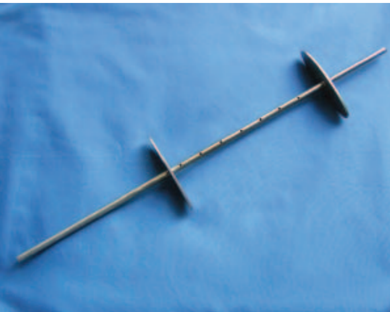
Figure 2. Typical cooker sampling probe
