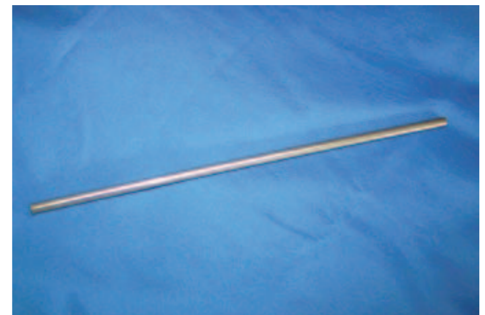
Figure 1. Typical openended sampling probe
