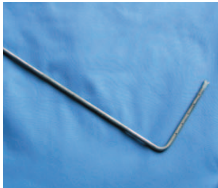
Figure 3. Typical angled multi hole sampling probe
